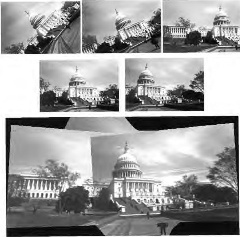
Fig. 19.3. Calibrating a camera rotating about its centre. (upper) Five images of the US Capitol acquired by approximately rotating the camera about its centre. (lower) A mosaic image constructed from the five images (see example 8.14(p207)). The mosaic image shows very clearly the distortion effect of the infinite homography between the images. Analysis of this distortion provides the basis for the auto-calibration algorithm. The calibration is computed as described in algorithm 19.3.
