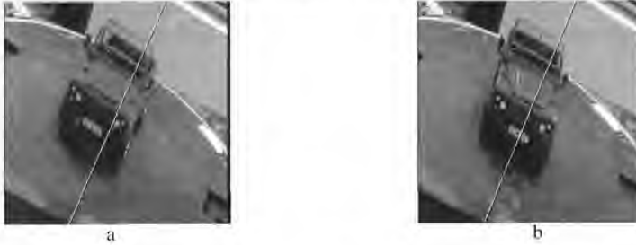
Fig. 14.14. Computing motion from affine epipolar geometry. (a)(b) Two views of a buggy rotating on a turntable. The computed rotation axis is superimposed on the image, drawn to pass through the image centre. The ground truth axis is, of course, perpendicular to the turntable in the world.
