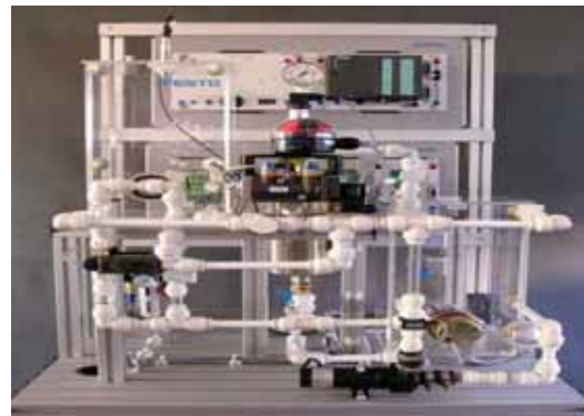
Figure 3. Hardware model of the Water level control unit
