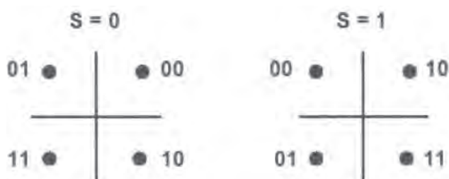
Figure 2-21: Cover code bit-to-symbol mapping in QPSK mode
