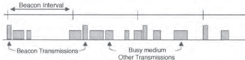
Figure 2–15: The beacon transmission is almost periodic
