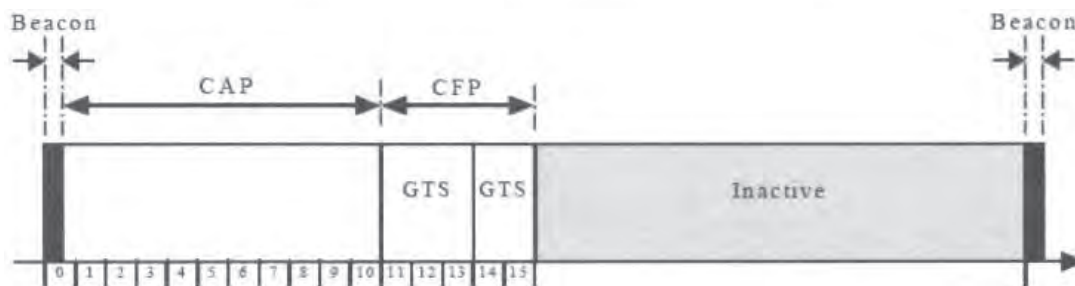
Figure 3-24: General superframe structure, with active and inactive periods
