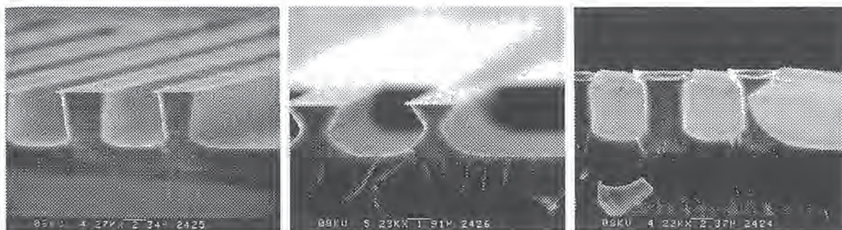
Figure 10: The influence of mask material on the profile. Left=copper. Mid=platinum. Right=aluminium.
