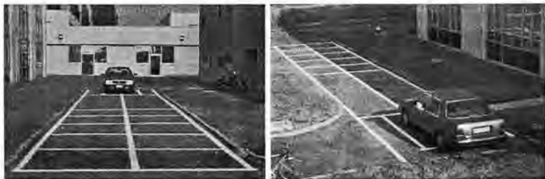
Fig. 6.2 View of the calibration grid painted on a reference road segment.
