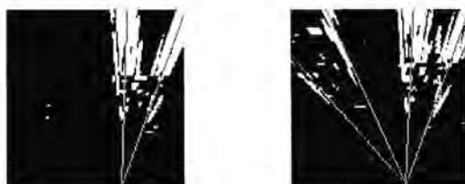
Fig. 4.32 Correspondence between triangles and directions pointed out by peaks detected in the polar histogram.
