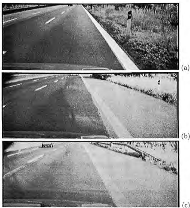
Fig. 8.2 The reflection problem: (a) image with no reflections; (b) image with a strong reflection; (c) over-saturated image due to reflections on the windscreen.
