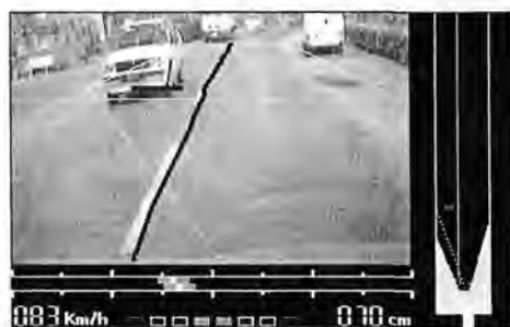
Fig. 6.6 The output of the GOLD system on the on-board monitor.
