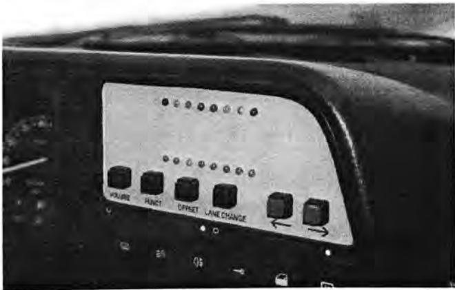
Fig. 6.3 The control panel, which includes the two sets of leds and a series of buttons.
