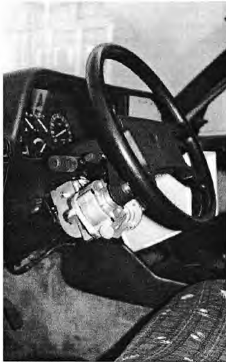
Fig. 6.8 View of the electric engine installed on the steering column.
