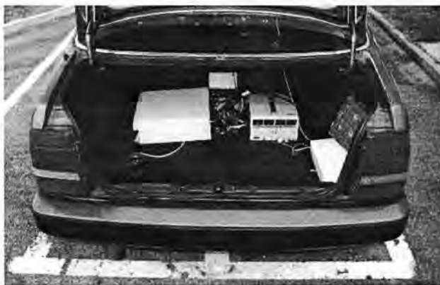
Fig. 6.4 Internal view of ARGO's boot: both the PC and inverter are visible.
