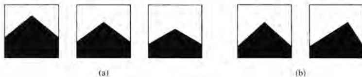
Fig. 4.1 Synthetic images used as road models for: (a) different camera positions and/or orientations (b) different number of lanes (assuming right-hand side driving).
