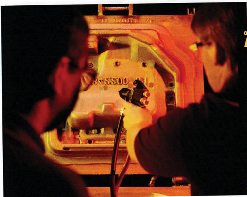
Figure 1 | The main way mold-release agents are applied to the mold is through the use of a spray gun. The nozzle is adjusted to ensure proper atomization and good film formation. [Courtesy of Chem-Trend LP]
