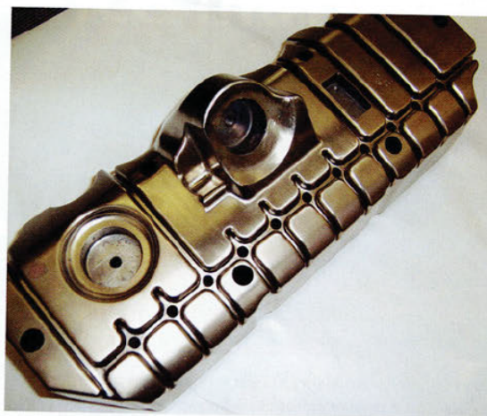
Figure 3 | One of the key properties of a mold coating is abrasion resistance. This is particularly important in applications such as this core section which is used to mold fiberglass material. [Courtesy of Bales Mold Service, Inc.]
