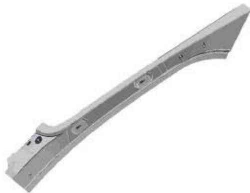
Figure 21 : C5 A frame reinforcement
