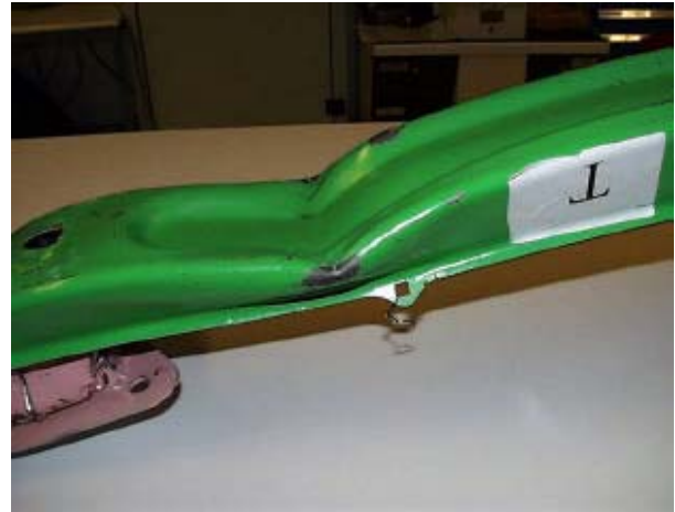
figure 23 : Front bumper beam of the LAGUNA II after urban crash
