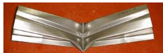
Figure 12 : Photo of a typical test piece after a dynamic, three-points bending impact test.
