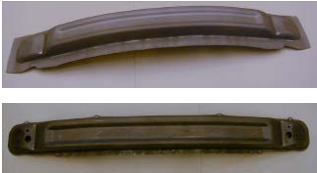
Figure 22 : LAGUNA II front bumper beam before and after cutting
