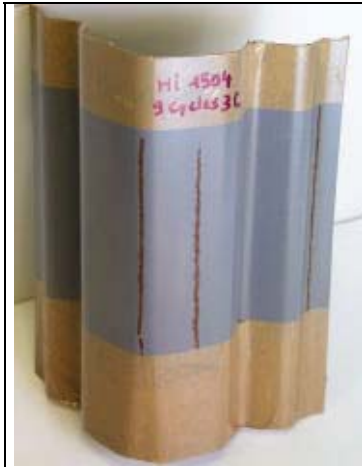
Figure 17 : Photo of a hot-formed part after 6 months' Scab-testing carried out at Fos/Mer.
