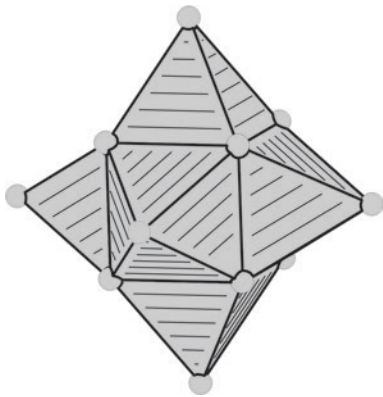
Fig. 3.79 The [\text{Ba}_{14}\text{CaN}_6] cluster unit in the structure of \text{Na}_{14}\text{Ba}_{14}\text{CaN}_6 . The calcium atom in the center of the cluster units belongs to each of the \text{N@Ba}_5\text{Ca} octahedra.
