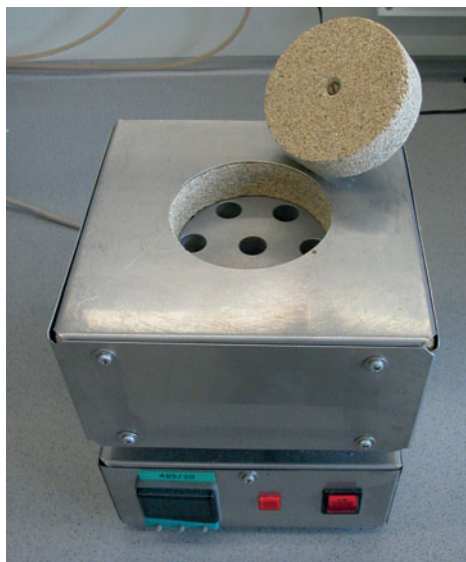
Fig. 2.7 Set-up of a home-made aluminum block furnace. For details see text.
