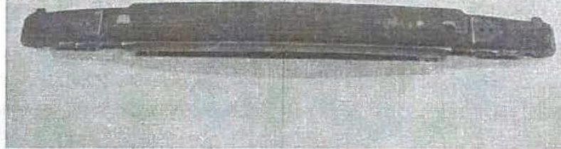
FRONT BUMPER BEAM OF THE CITROËN C5 USIBOR 1500 PRECOATED IN 1.5 mm THICKNESS (BEFORE CATAPHORESIS) (PHOTO WITH THE KIND PERMISSION OF PSA PEUGEOT CITROËN)
