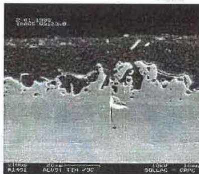
SECTION OF ALLOYED AND CATAPHORIC LAYER BY SEM IN BSE MODE
