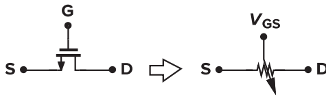
Figure 2.13 MOSFET as a controlled linear resistor.
