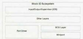
Figure 29. The architecture of the block I/O subsystem
