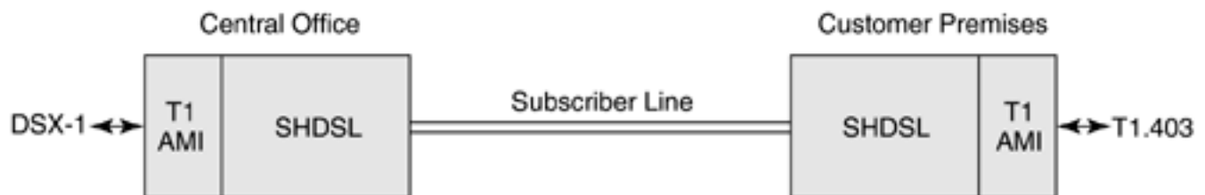
Figure 6.1. T1 extension application.
