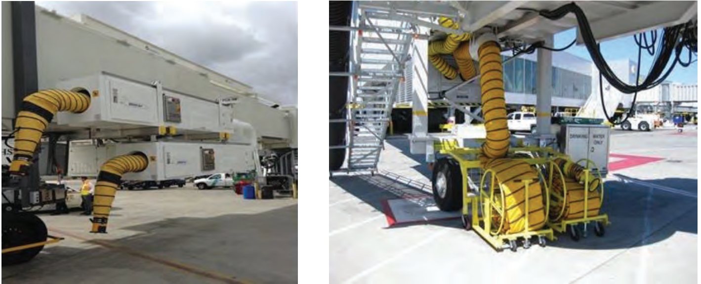
Figure 15. Twist Aero's Boom-Air Hose Management System (left). ITW GSE PCA hose reel with extension reels (right) (Source: Twist Inc. and ITW GSE).
