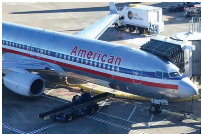
Figure 23. Aircraft connected to electric PCA and 400 Hz ground power (left) and PCA hose and basket (right) (Source: Katherine Preston, Harris Miller Miller & Hanson, Inc.).
