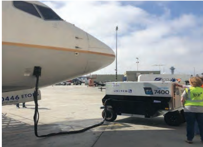
Figure 6. Mobile battery-powered GPU, ITW GSE Model 7400 (Source: ITW GSE).
