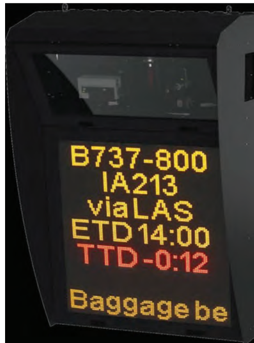
Figure 14. Typical ramp information display system (Source: Frederick Roe, ADB Safegate).
