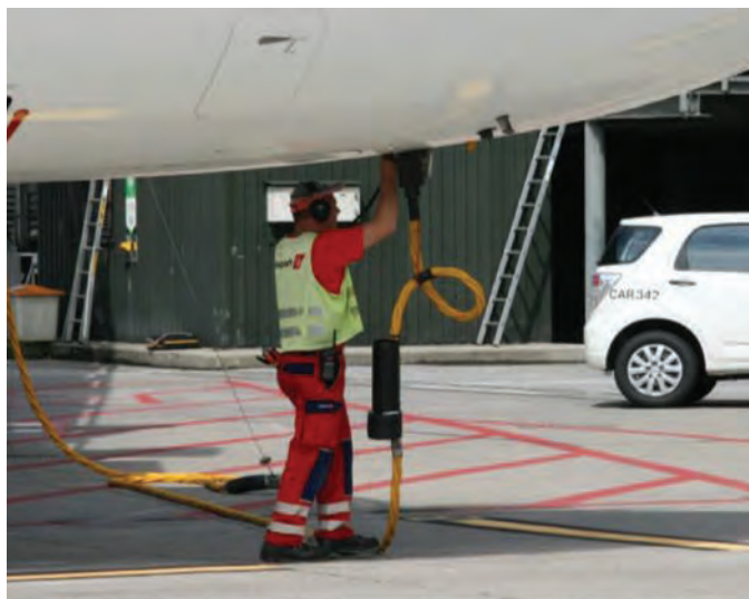
Figure 40. Ground crew plugging in power cable (Source: Zurich International Airport).
