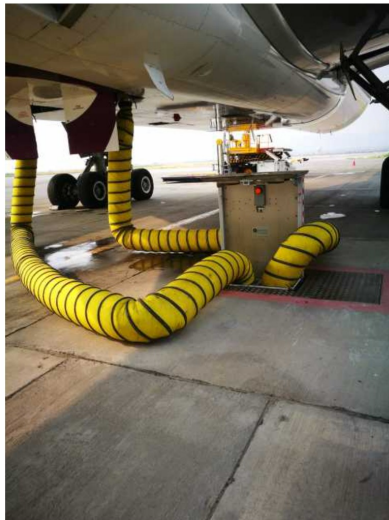
Preconditioned Air (PCA) Hose connects with aircraft PCA receptacle to establish a ground service connection and pump air into the air distribution network of aircraft
