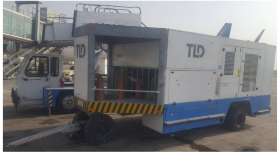
A mobile PCA unit is simply a PCA unit in which all components have been assembled over a cart that can be towed to any desired location
