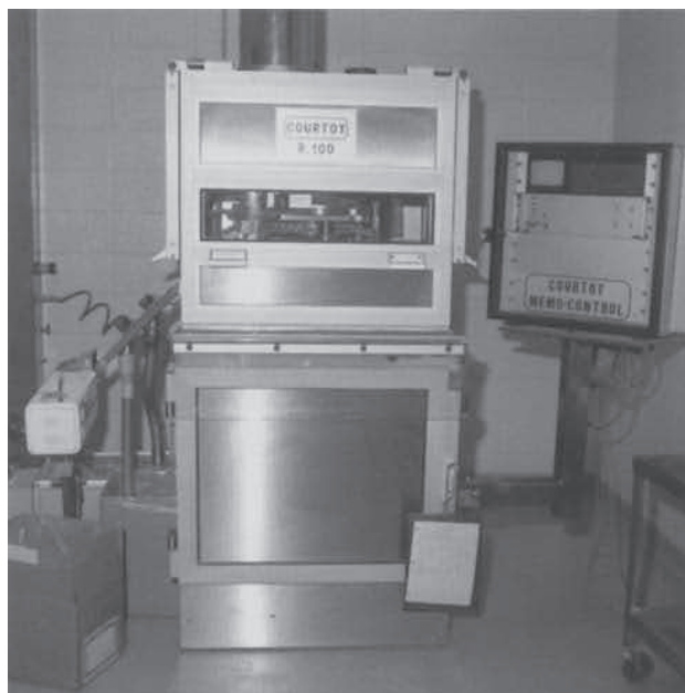
Figure 45-27. Courtoy R-100 with computer-controlled operation.
