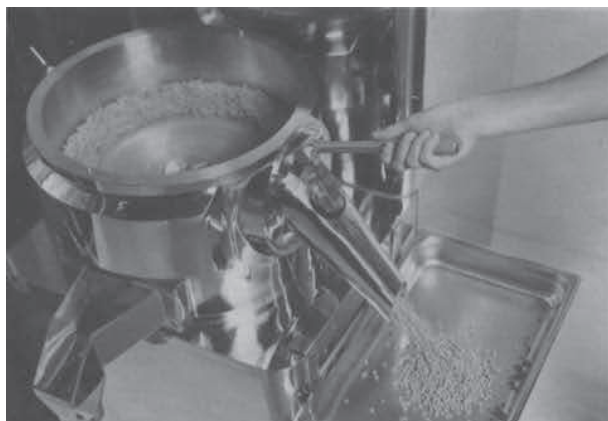
Figure 45-15. The inside of a QJ-400 Marumerizer (courtesy, Luwa).
