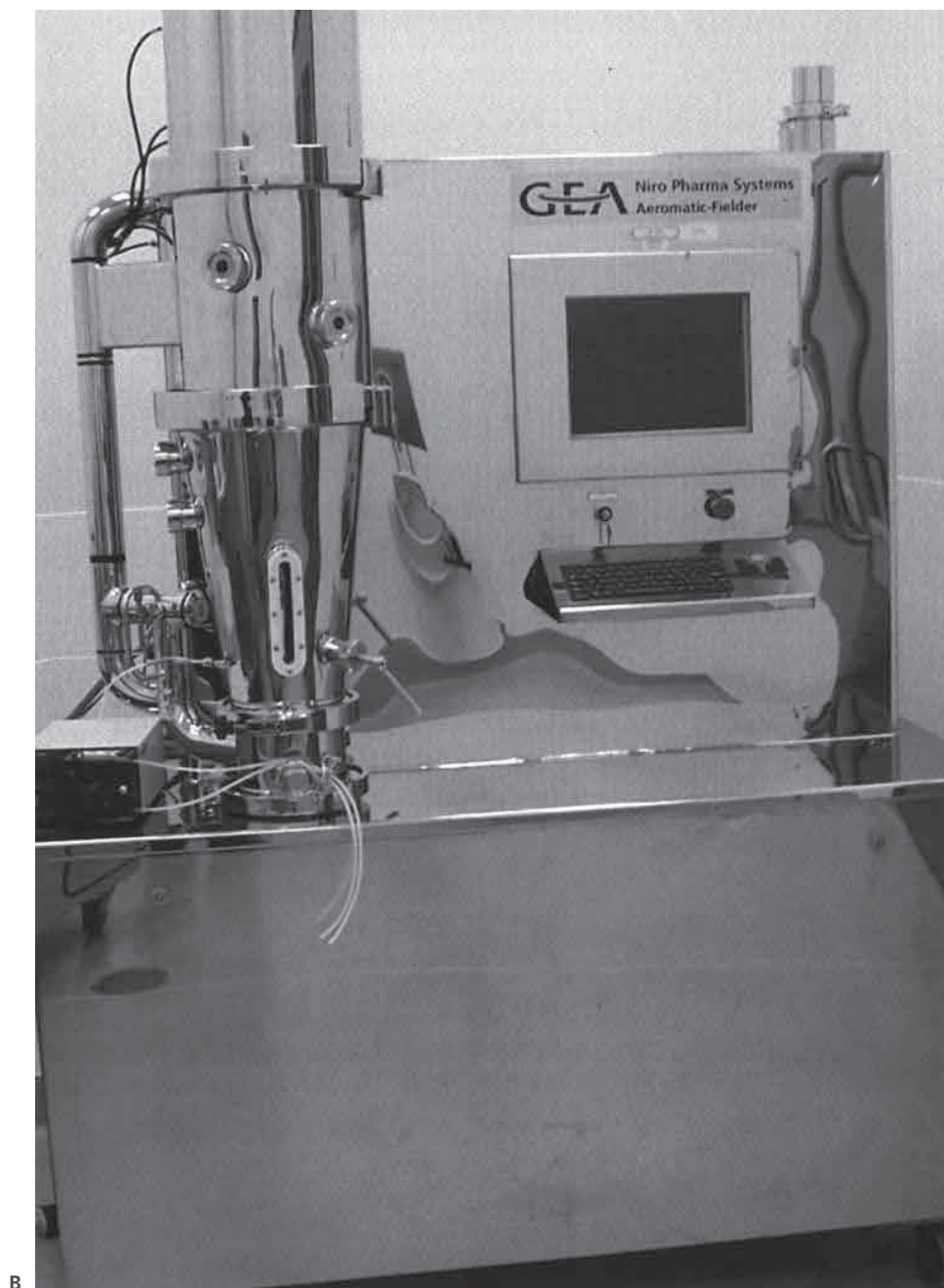
Figure 45-13. (continued) b. Computer-controlled/monitored coating.
