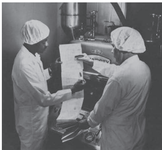
Figure 45-1. Tablet press operators checking batch record in conformance with Current Good Manufacturing Practices (courtesy, Lilly).
