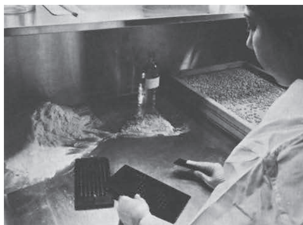
Figure 45-33. Hand-molding tablet triturates (courtesy, Merck).
