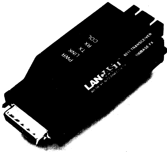
FIGURE 3.9 Fast Ethernet MII transceivers are similar to the old Ethernet AUI transceivers, but are very rare because most Fast Ethernet hardware includes an onboard transceiver. MII uses a 40-pin connector very similar to SCSI-2.
