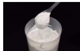
Titanium oxide (viscosity: 5,300mPa·s, 50wt%)
