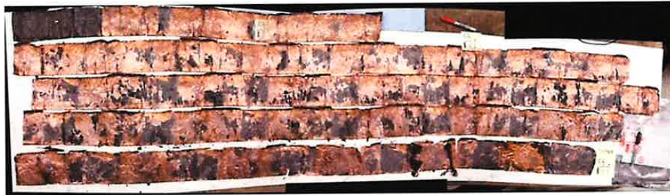
Figure 14. Cell 6 winding closest to cell 5.
