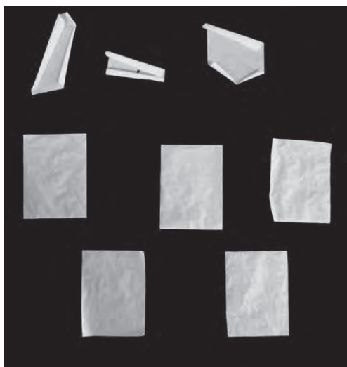
Fig. 2. Photographs of PE membranes and ceramic-coated separators (ACS-3) after being kept at 105 °C for 1 h.
