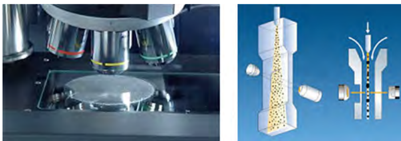
Figure 18: Illustration of static imaging (left) and dynamic imaging (right) optical arrangements.
