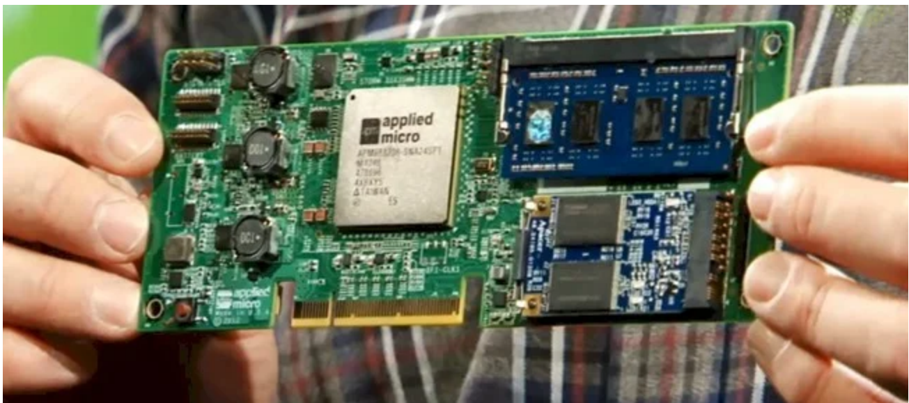
An X-Gene ARM microserver that plugs into the Group Hug backplane
