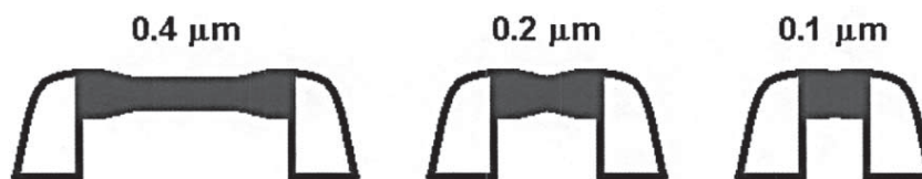
FIGURE 59. Schematics of the reversed fine-line effect for \text{CoSi}_2 (due to Co diffusion in \text{Co}_2\text{Si} ) and NiSi formation.
