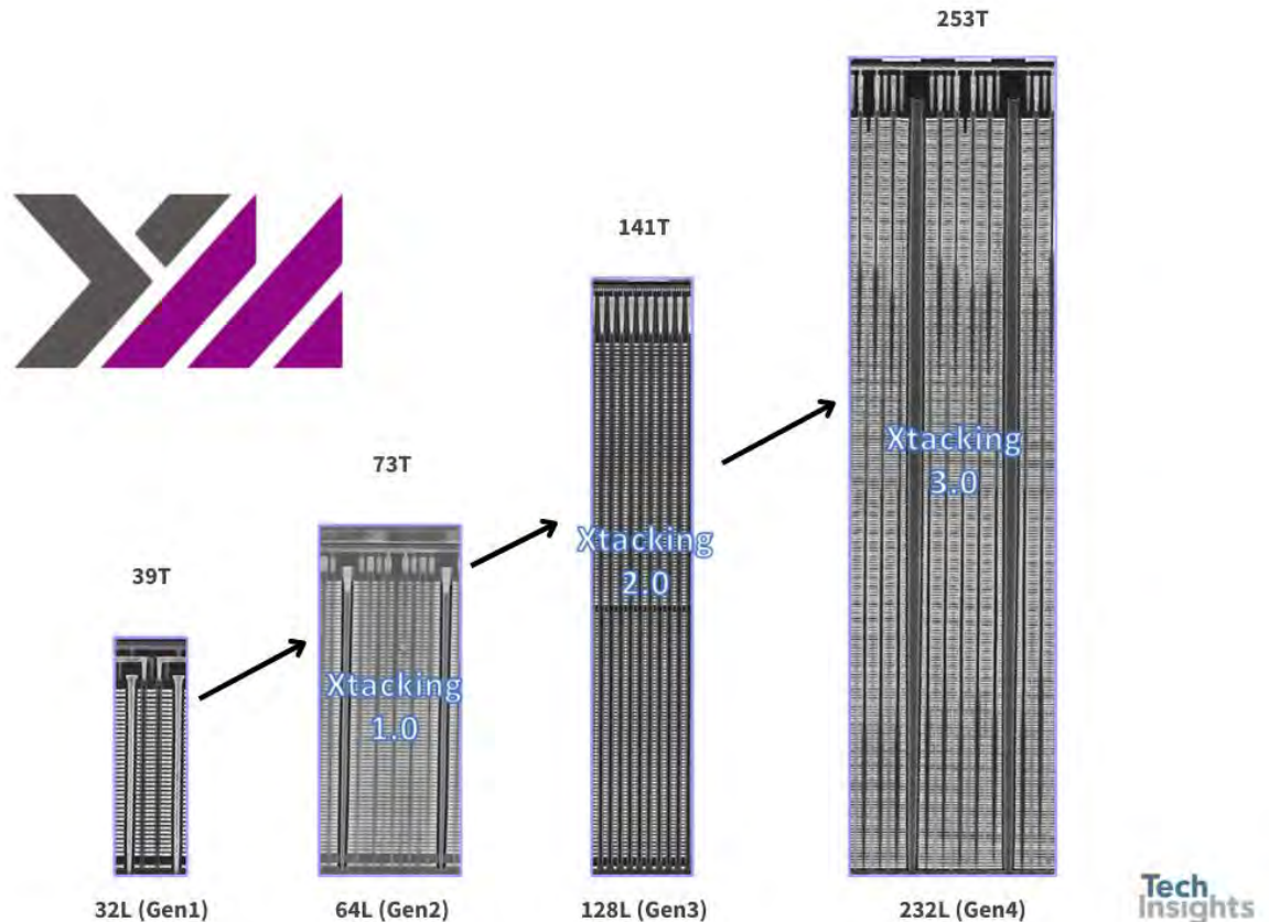
Figure 3. YMTC 3D NAND cell structure, Gen1 32L through Gen4 232L (x-sectioned SEM images in BL direction), TechInsights 2022
