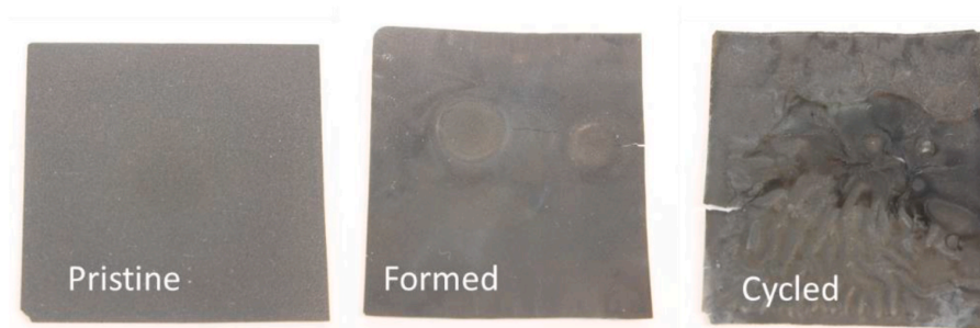
Fig. 4. Photographs of the delaminated pristine, formed, and cycled LCO cathodes (approximate size 2.5 cm × 2.5 cm) showing mechanical damage increase as the cell cycles.
