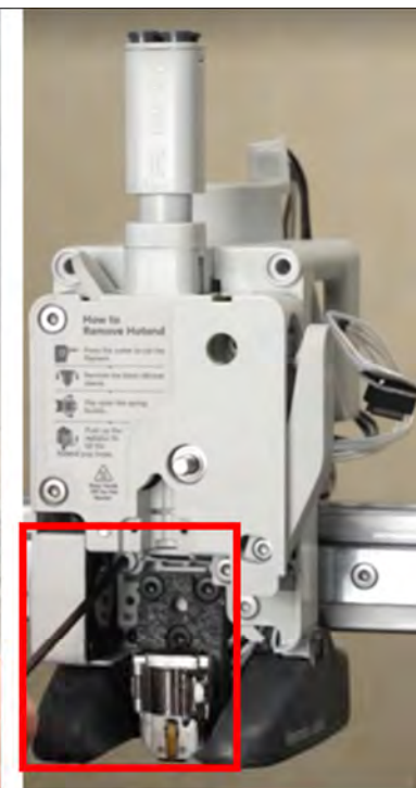
Hotend heating assembly and fan
