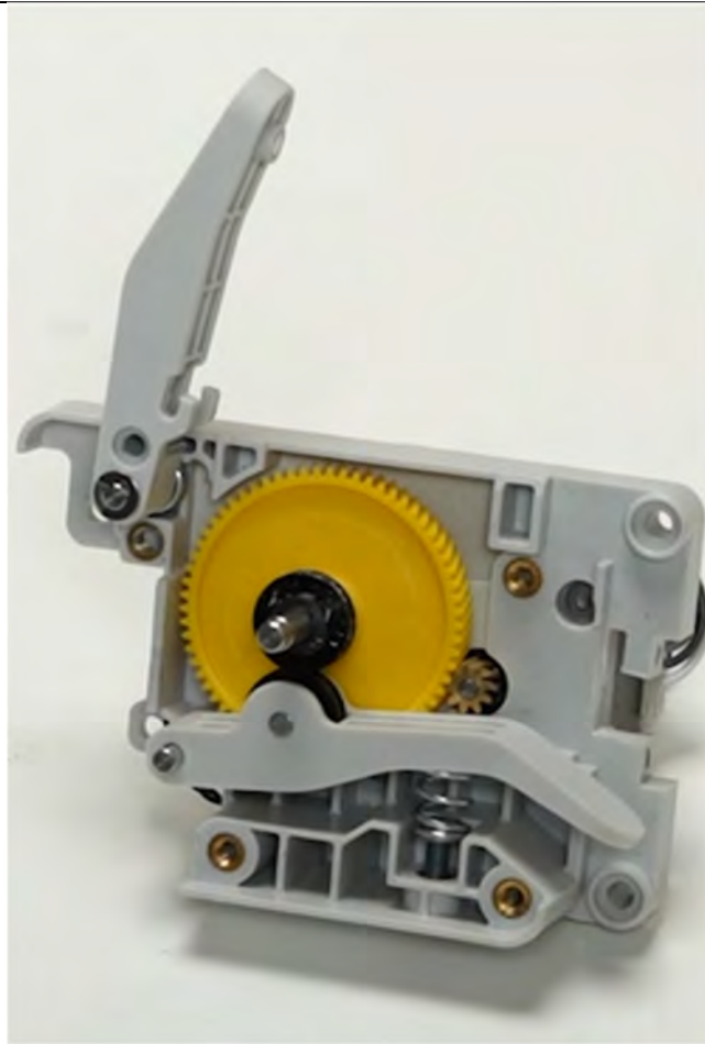
Internal Gear Structure of the Extruder
