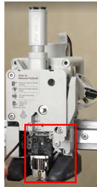
Hotend heating assembly and fan
