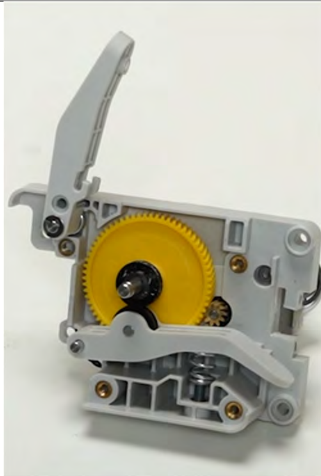
Internal Gear Structure of the Extruder
