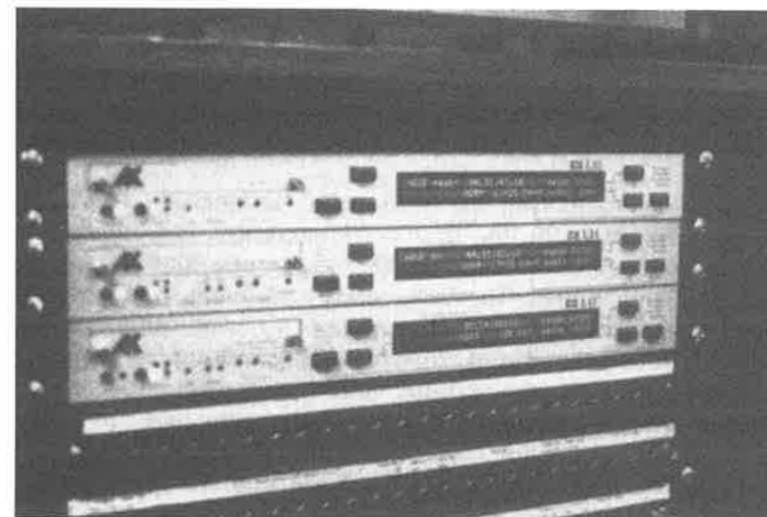
Figure 9.6 Audio Kinetics ESbus synchronizers. The top module is the master.
