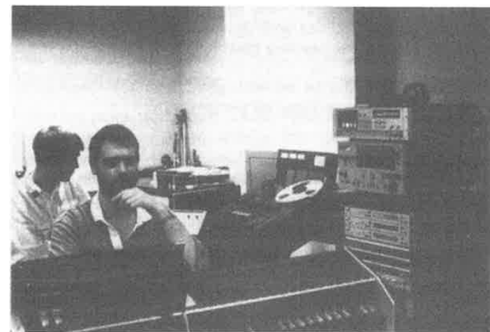
Figure 9.7 ESbus synchronizers controlling multi-track and R-DAT machines from a VCR master during audio post-production.
