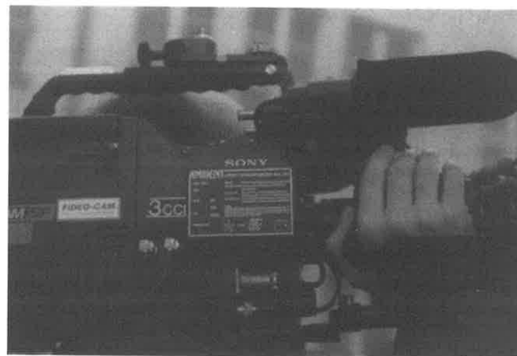
Figure 8.15 A commercially available highly stable timecode and video syncs generator. It can be jammed to a Master and its stability can be checked. Courtesy Ambient Recording GmbH.
