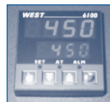
Figure 5 Temperature controller. The upper display is the controlled variable and the lower is the setpoint.
