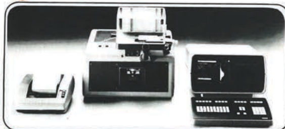
The photograph shows one of Fischer's latest developments: the Fischerscope X-Ray 1000.
