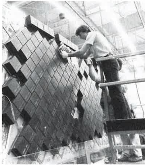
FIGURE 23.17 Photograph showing the installation of thermal protection ceramic tiles on the Space Shuttle Orbiter. [Photograph courtesy the National Aeronautics and Space Administration (NASA).]
