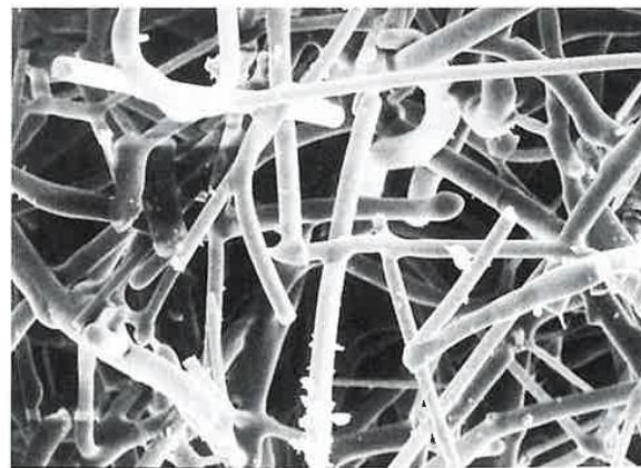
FIGURE 23.18 Scanning electron micrograph of a Space Shuttle Orbiter ceramic tile showing silica fibers that were bonded to one another during a sintering heat treatment. 750×. (Photograph provided courtesy of Lockheed Aerospace Ceramics Systems, Sunnyvale, California.)
