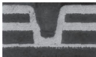
FIGURE 29.5 Horizontal PTH/pulse-plated microvia.
