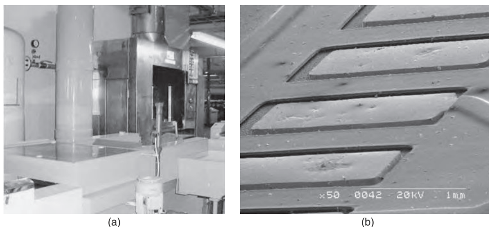
FIGURE 32.2 (a) HASL equipment (b) surface scanning electron micrograph (SEM).
