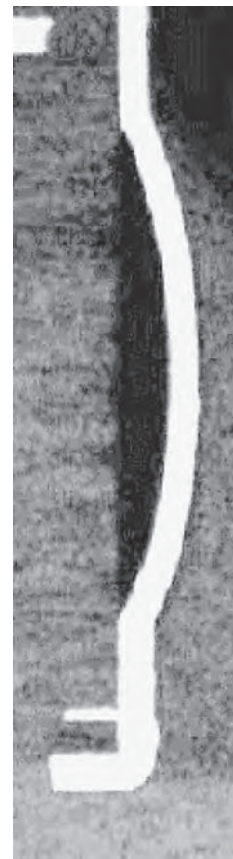
FIGURE 27.43 Hole wall pull-away.
