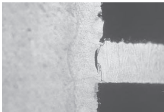
FIGURE 51.22 Resin Smear in PTH, vertical microsection. (Courtesy of IPC.)
