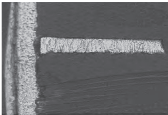
FIGURE 51.30 Interconnection separation, vertical micro-section. (Courtesy of Microtek Laboratories.)
