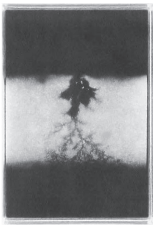
FIGURE 57.10 Transmitted light micrograph through a PCB that failed in the field. Dendritic growth has formed at the interface of a UV-cured screened solder mask and the FR-4 surface.
