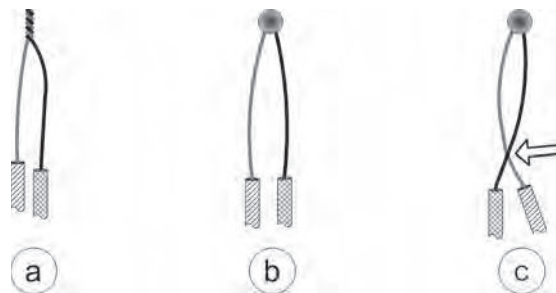
FIGURE 47.10 Thermocouples: (a) twisted couple; (b) welded couple; (c) welded couple with an inadvertent couple (see arrow).
