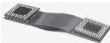
FIGURE 65.2 Air gap structure of multilayer rigid-flex board.
