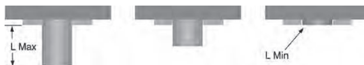
FIGURE 52.30 Lead protrusion violates minimum clearance requirements. Lead protrusion exceeds maximum design height requirements. (IPC)
