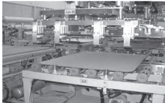
FIGURE 6.11 Automated build-up of copper and prepreg.
