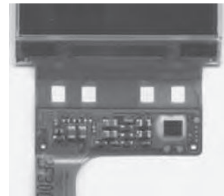
FIGURE 65.15 Rigid/flexible circuit for LCD driver.
