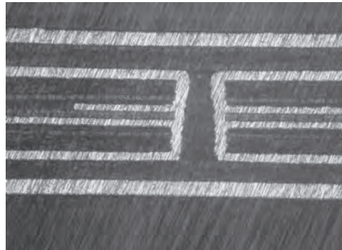
FIGURE 65.16 Micro inner vias in multilayer rigid/flexible circuit construction.
