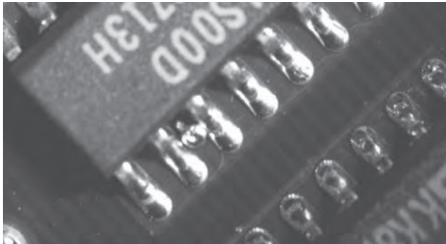
FIGURE 52.24 Solder ball causing a short circuit between pins in SOIC.
