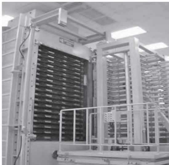
FIGURE 6.14 Lamination press with multiple openings. (Photo Courtesy of Polyclad Laminates, Inc.)
