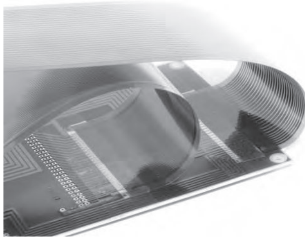
FIGURE 64.5 Flexible circuits connected to a rigid board by solder fusing.
