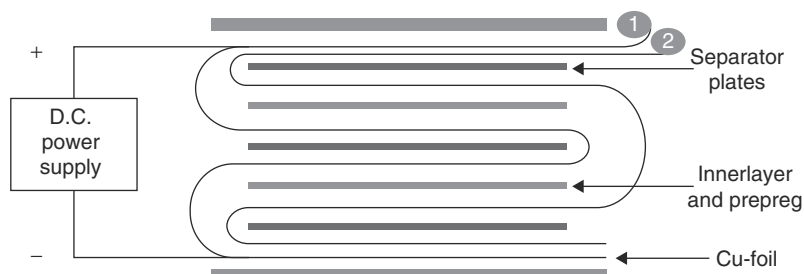
FIGURE 6.15 Laminate pressing with continuous copper foil and direct current heating. (Illustration Courtesy of Cedral)
