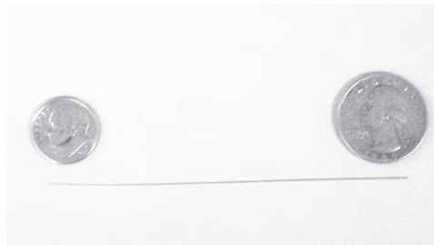
FIGURE 39.1 Tapered pin for a fine-geometry fixture.
