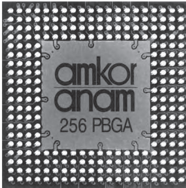
FIGURE 13.11 Typical ball grid array package. (Courtesy of Icon Industries.)
