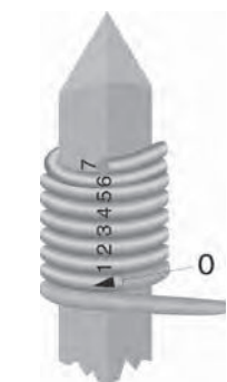
FIGURE 52.36 Solderless wire wrap acceptability. (IPC)
