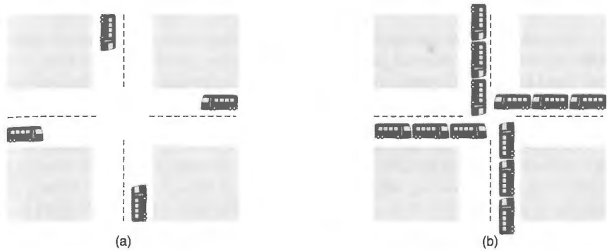
Figure 1-13. (a) A potential deadlock. (b) An actual deadlock.
