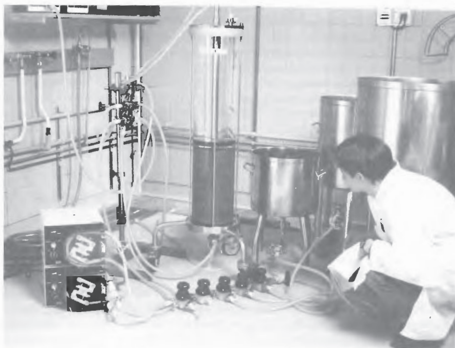
FIGURE 1-4. Setup of an expanded bed adsorption experiment using a 200-mm-diameter STREAMLINE column. The column is supplied with STREAMLINE rProtein A for the capturing of monoclonal antibodies directly from a whole hybridoma cell culture. (Courtesy of Pharmacia Biotech AB, Uppsala, Sweden.)
