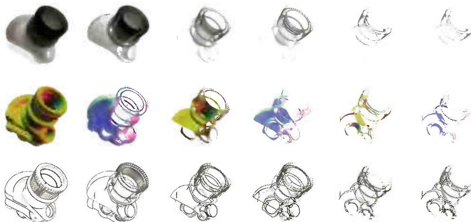
Figure 15-2. The Z-Buffer, Normal Buffer, and Edge Map for Each Layer
