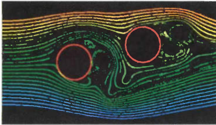
Figure 47-8. Particles Advected in a 2D Flow Field Based on the D2Q9 LBM Model
