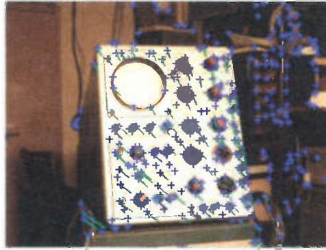
Figure 40-5. Detecting Distinctive Points as the Camera Pans The GPU is used to detect and track distinctive points (features) in real time as the camera pans. The green lines connect the same point in the previous image to its new location in the current image.
