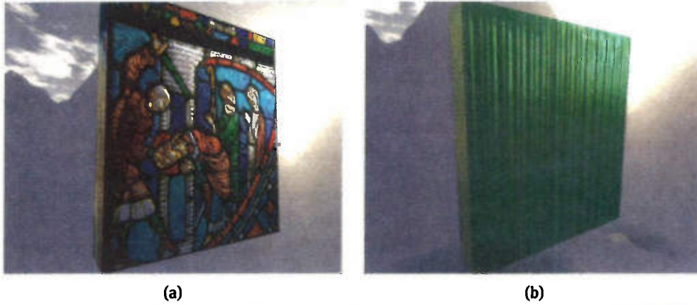
Figure 19-8. Different Glass Types (a) Stained glass. (b) Partition glass.
