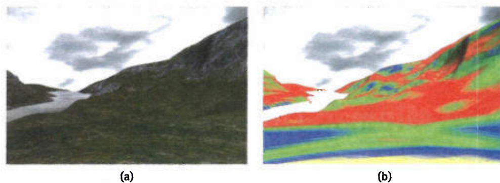
Figure 28-1. Applying a False-Colored Mipmap to a Terrain (a) Terrain rendered using Climax's Leviathan engine. (b) The effect of substituting the false-colored mipmap from Figure 28-3. Note that the highest level (yellow) is barely visible.
