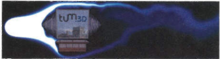
Figure 44-9. A Navier-Stokes Fluid Dynamics Simulation On a 512 \times 128 grid running at 110 frames/sec, including rendering time.
