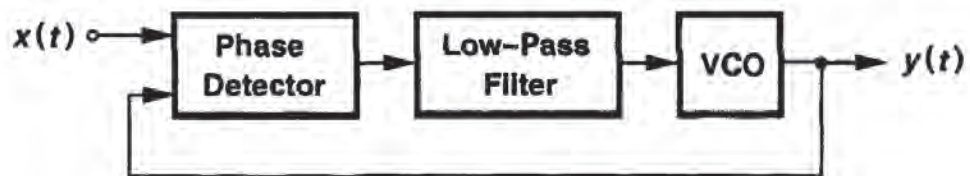
Figure 8.8 Basic phase-locked loop.
