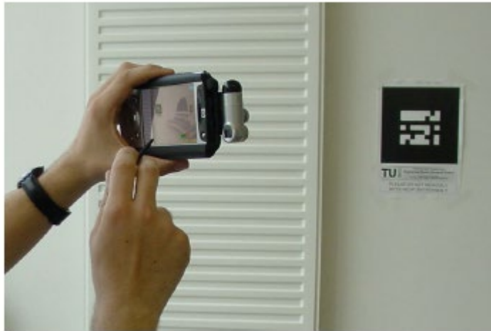
Figure 1. The self-contained handheld AR system can track optical markers in real time.
