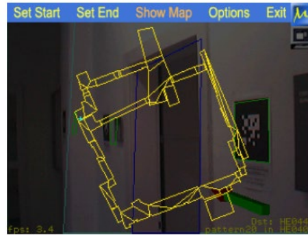
Figure 8. Signpost showing the overview map (current user position marked with small cross)
