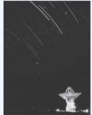
FIGURE 1.7 The search for extraterrestrial life is being carried out with radio antennas like the one pictured here. A radio antenna is an example of a system with position controls
