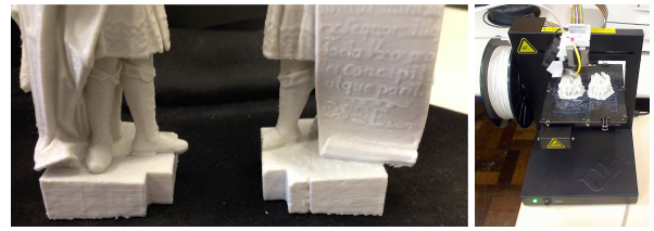
Fig. 4. Scaled restoration of left foot of the prophet Hosea (left sculpture) compared to the original scanned model (right sculpture). Models were printed in PLA.
