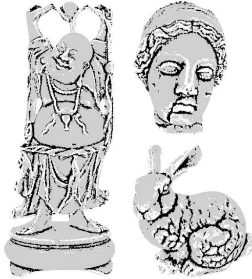
Figure 11: Salient curvature extrema triangles detected on complex triangular meshes.
