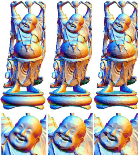
Figure 2: Left: Stanford Buddha statue consisting of 1,087,716 triangles. Middle and right: simplified meshes consisting of 17,400 triangles (98.4% reduction). Middle: decimation according to the Garland-Heckbert quadric error metric method. Right: modified Garland-Heckbert method was used.
