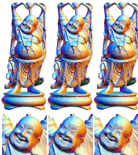
Figure 2: Left: Stanford Buddha statue consisting of 1,087,716 triangles. Middle and right: simplified meshes consisting of 17,400 triangles (98.4% reduction). Middle: decimation according to the Garland-Heckbert quadric error metric method. Right: modified Garland-Heckbert method was used.
