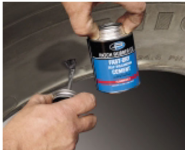
Brush on cement.
