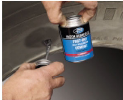
Brush on cement.
