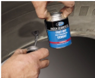
Brush on cement.
