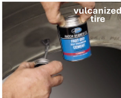
Brush on cement.
