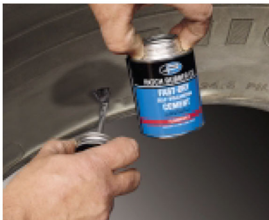
Brush on cement.
