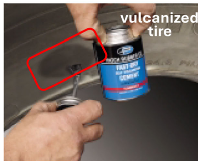
Brush on cement.
