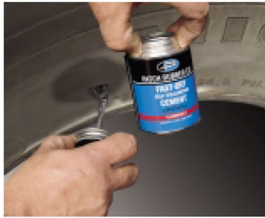
Brush on cement.
