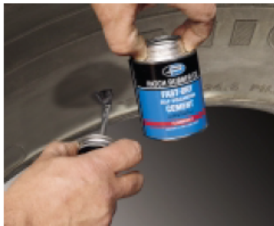
Brush on cement.
