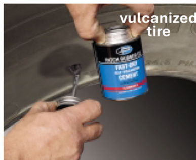
Brush on cement.
