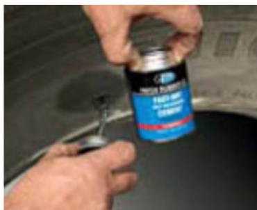
Brush on Cement
