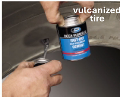
Brush on cement.
