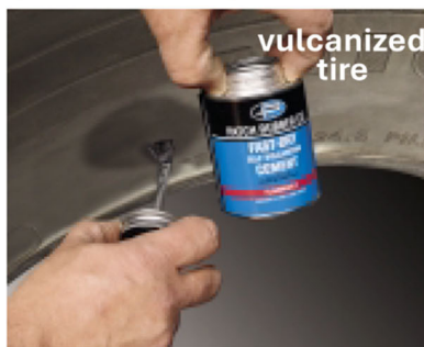
Brush on cement.
