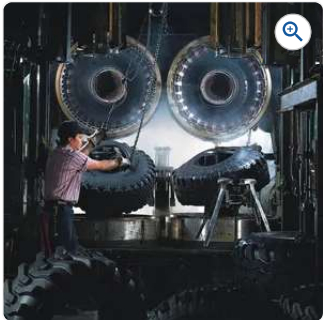
truck tires being removed from their molds
