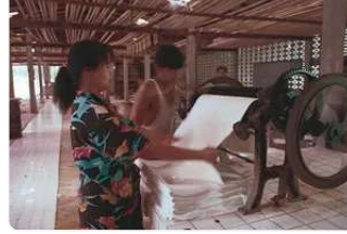
sheets of natural rubber coagulated from latex being passed between rollers Sheets of natural rubber coagulated from late...(more)
