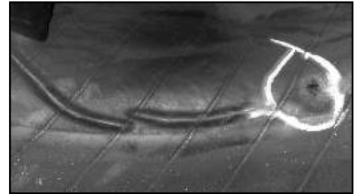
This photo shows innerliner separation in a run flat tire. The tire should not be repaired if this condition is present.
