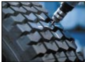
From the outside of the tire ream the injury using the carbide cutter with a 6491QR slow speed buffer.
