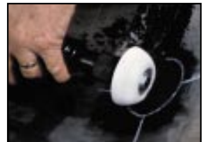
Buff the repair area using a buffing or contour wheel with the slow speed buffer.
