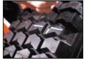
Inspect the damage using a 190 awl.
