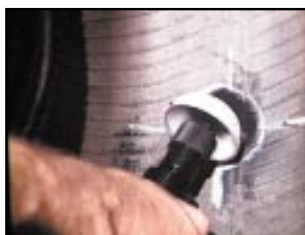
Buff the repair area using a buffing or contour wheel with the slow speed buffer.
