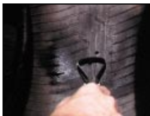
Use a #28 scraper to remove contaminates.
