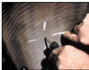
Inspect the damage using a 190 awl
