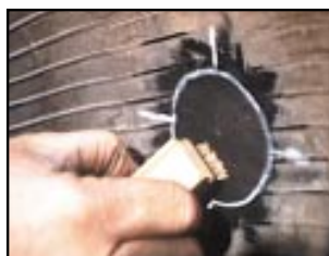
Using the 6014 Brass Brush, remove the buffing dust from the buffed area.
