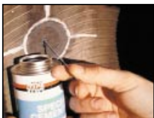
Using Special Blue Cement and a 626 pull wire, cement the injury channel.
