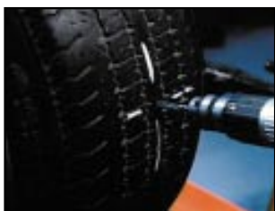
From the outside of the tire ream the injury using the carbide cutter with a 6491QR slow speed buffer
