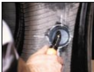
After the repair unit is applied, stitch thoroughly from the center out
