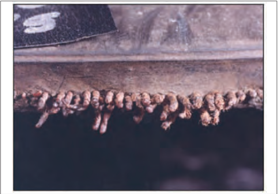
Figure 15.15: Broken, heat-fused polyester body cords, upper sidewall
