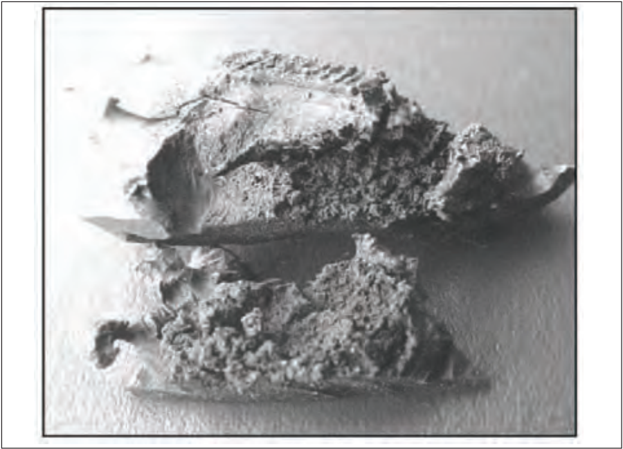
Figure 15.7: Examples of reverted tread rubber
