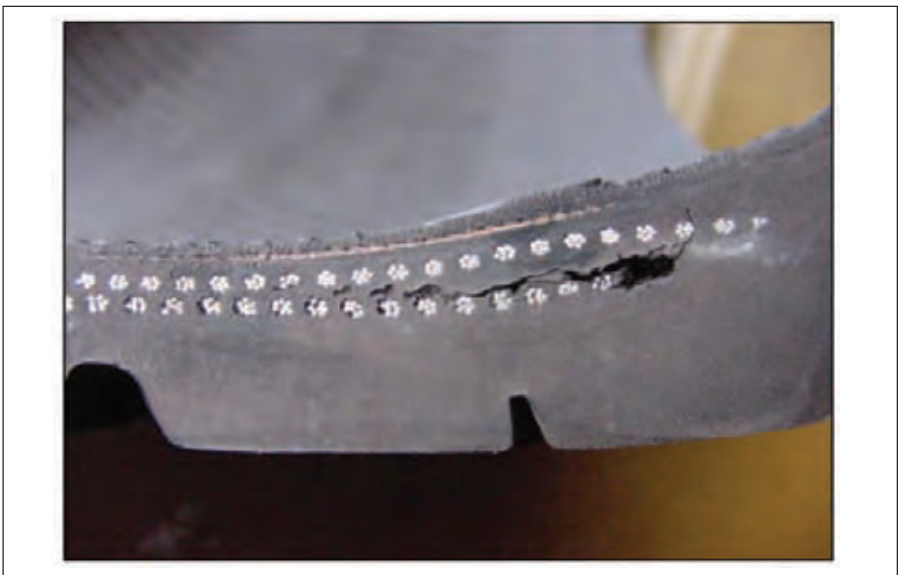
Figure 15.13: Cracking between steel belt edges
