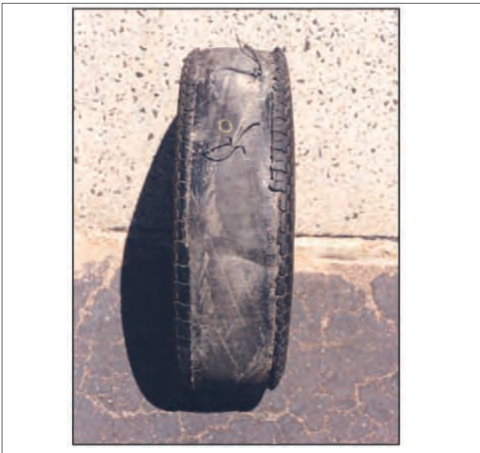
Figure 15.16: Exemplar tire after tread/belt detachment
