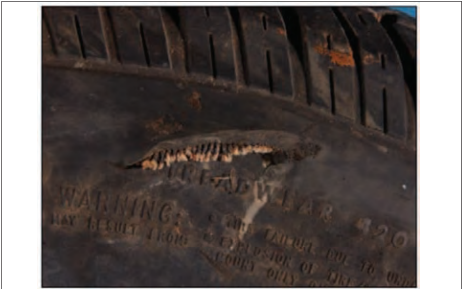
Figure 15.17: Upper sidewall break through to cavity
