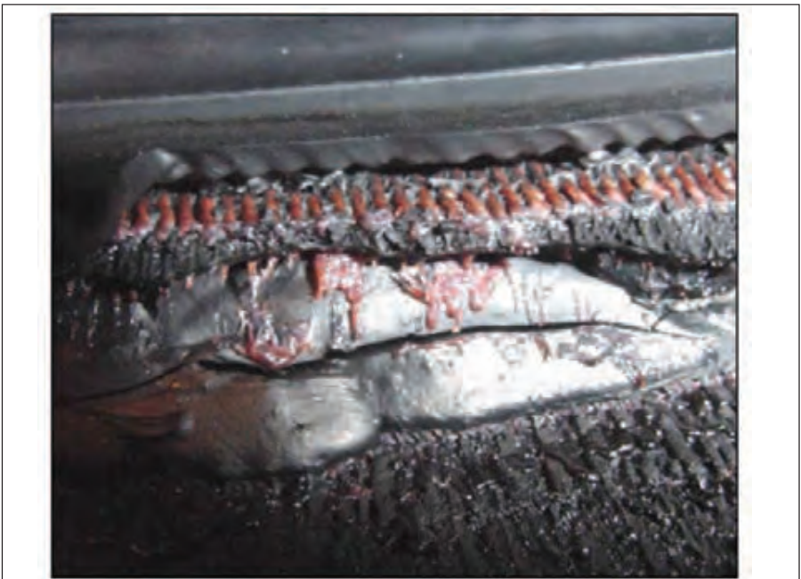
Figure 15.8: Melted polyester cord (lower sidewall)
