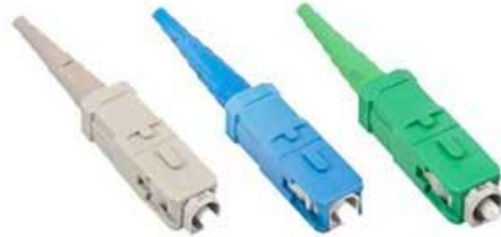
Connector color codes: L>R, Multimode, Singlemode, SM APC
