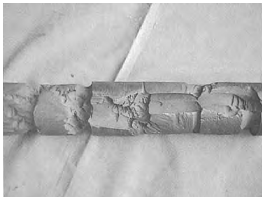
FIGURE 22 The corrosion erosion of a carbon steel shaft that was damaged in an ultra-pure water service after approximately 6 months
