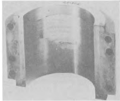
FIGURE 25 Bearing wipe on a 3-in (76-mm) diameter bearing due to temporary loss of lubricant (Westinghouse Electric Corp. Photo originally reproduced in Ref. 8, p.18–25 )
