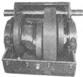
FIGURE 18 A cast crankshaft with integral gear (Continental-EMSCO)
