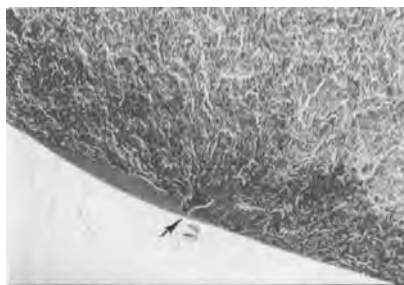
FIGURE 18 SEM photo of a fatigue smooth fatigue test specimen with a single origin. The arrow indicates the fatigue crack origin.
