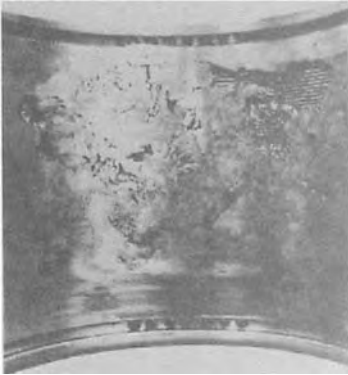
FIGURE 24 Babbitt fatigue in a 7-in (178-mm) diameter turbine bearing (Westinghouse Electric Corp. Photo originally reproduced in Ref. 8, p.18–19. )
