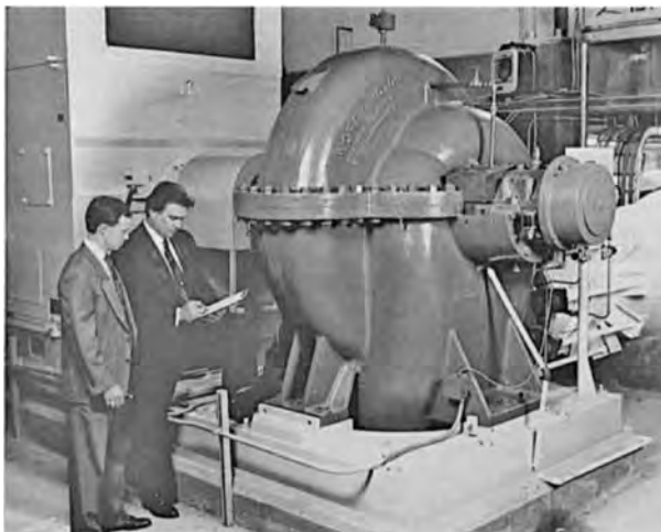
FIGURE 14 A bottom-suction, axially split casing single-stage pump (Flowserve Corporation)
