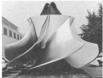
FIGURE 4 Mixed flow propeller runner (Voith Siemens Hydro)
