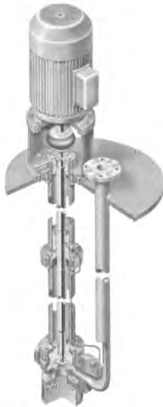
FIGURE 88 A vertical wet-pit volute pump with open shafting, no seal chamber (stuffing box), and its own thrust bearing (Flowserve Corporation)
