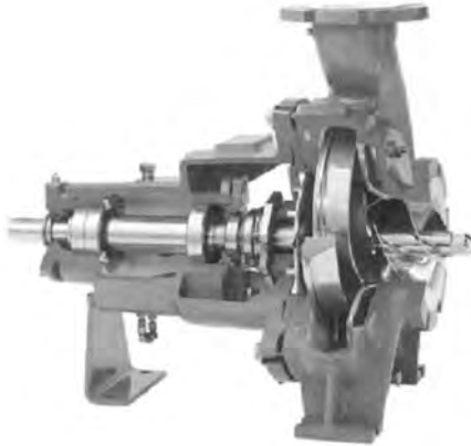
FIGURE 27 A centrifugal pump with a conventional impeller preceded by an inducer (Flowserve Corporation)
