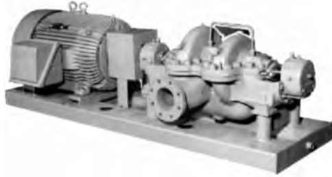
FIGURE 18 Two-stage axially split casing volute pump for pressures up to 500 lb/in 2 (34 bar) (Flowserve Corporation)
