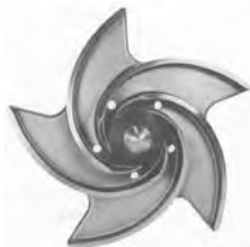
FIGURE 32 Open impeller with scalloped back shroud walls to reduce axial pressure unbalance (Flowserve Corporation)
