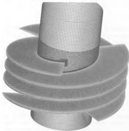
FIGURE 12 NASA 6-degree flat-plate inducer, tested in water and in liquid hydrogen at various temperatures at the NASA Glenn facility between 1964 and 1970.
