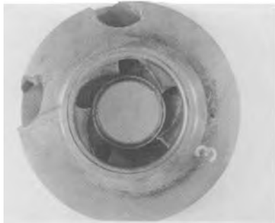
FIGURE 20 Overall view of a CF-3M impeller that has two corrosion-assisted fatigue fractures in the front shroud wall
