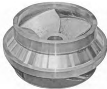
FIGURE 24 Medium specific speed, Francis vane radial impeller (Flowserve Corporation)
