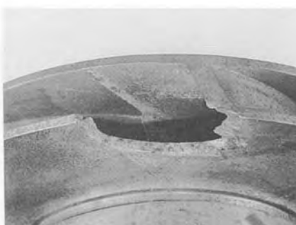
FIGURE 21 A higher magnification of one of the fatigue fractures that originated at a corrosion pit at the exit vane tip and shroud intersection. Additional corrosion pitting can be seen on the impeller in this figure.
