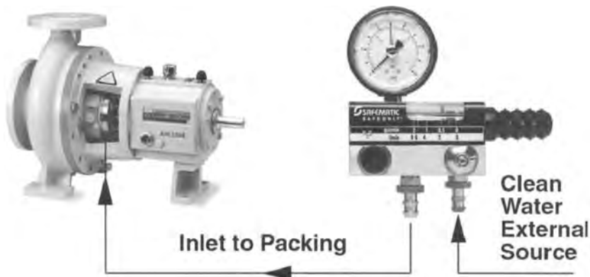
FIGURE 12 A regulation valve that controls and monitors the flow of water to the packing (Safematic)
