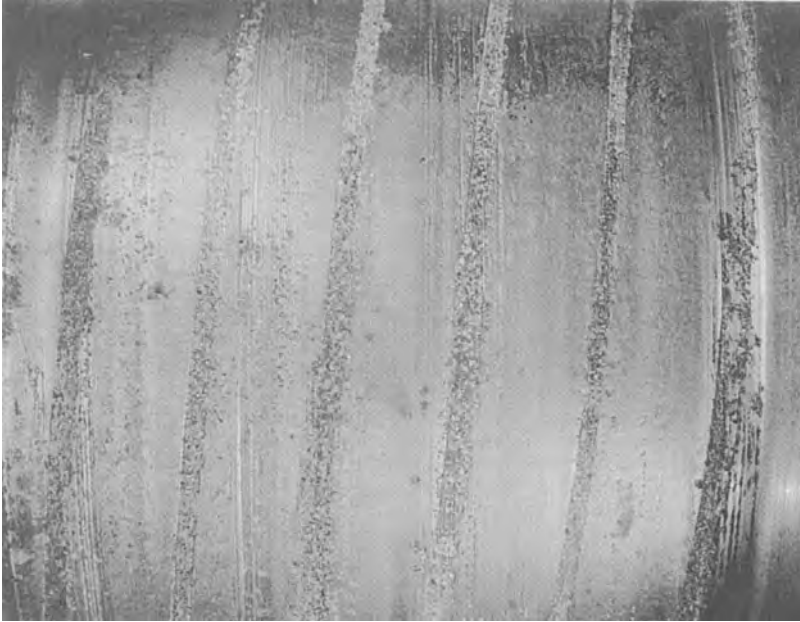
FIGURE 11 The three-body abrasive wear of a laser-hardened shaft sleeve in an abrasive service. Note the fine concentric scoring of the hardened surface. The helix pattern is the laser-beam overlapped zone produced by the laser process.
