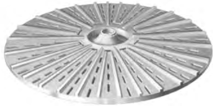
FIGURE 30 Barske-type radial multiple-vane open impeller with multiple balance holes to reduce axial pressure unbalance (axial thrust) (Flowserve Corporation)
