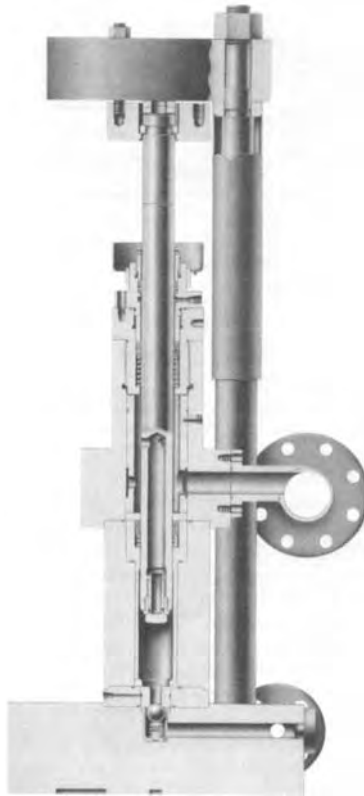
FIGURE 5 Special high-pressure liquid-end designs arrange the suction and discharge valves on the same axis as the plunger, thus eliminating intersecting bores (Flowserve Corporation).
