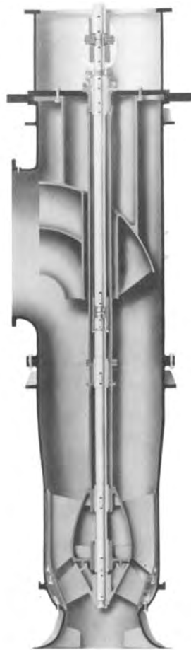
FIGURE 84 Vertical pull-out design allows the rotating element and critical non-rotating wear components to be removed for inspection and replacement without removing the complete pump (Flowserve Corporation)
