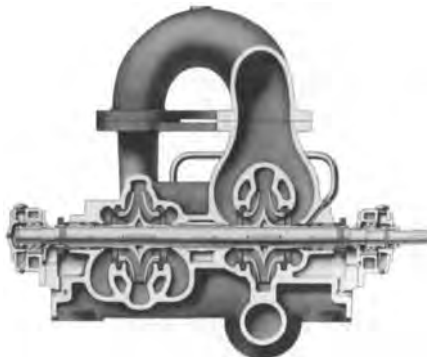
FIGURE 19 A two-stage double-suction, axially split volute pump with an external interstage passage bolted to the casing (Flowserve Corporation)
