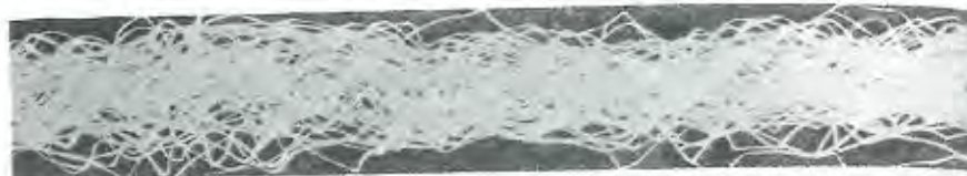
Figure 12.38. Texturalized 2-ply 70 den-34 filament yarn.
