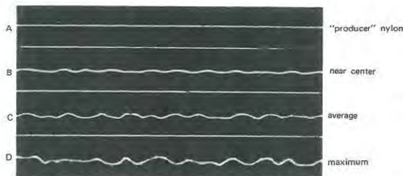
Figure 12.8. Longitudinal views of filaments from a 70 den/32 fils, nylon yarn, showing the differences in crimp due to the radial position in the yarn. A filament from untextured yarn; B, near center; C, middle layer; D, near the surface.
