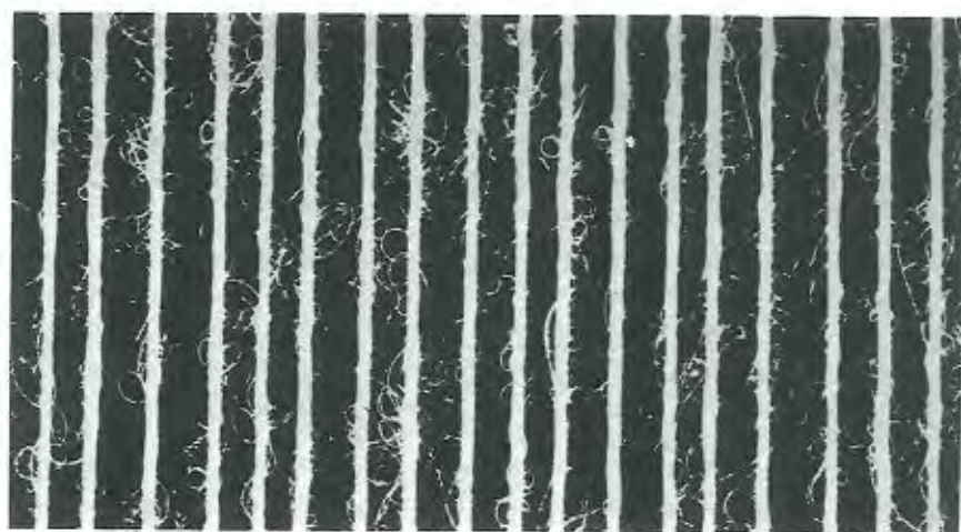
Figure 12.42(b). Photomicrograph showing fine-denier, multifilament Taslan textured nylon yarns. (courtesy E. I. Du Pont de Nemours & Company, Inc.).
