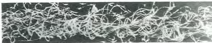
Figure 12.3. View of a typical stretch nylon yarn textured by the conventional twist-heat set-untwist technique.
