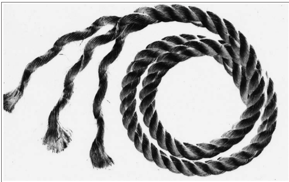
Figure 3.1: Hemp rope illustrating cord construction - filament/yarn/cord (rope)
