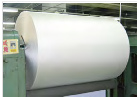
Tuck-in loom for tire cords Freshly woven product (whole cloth)
